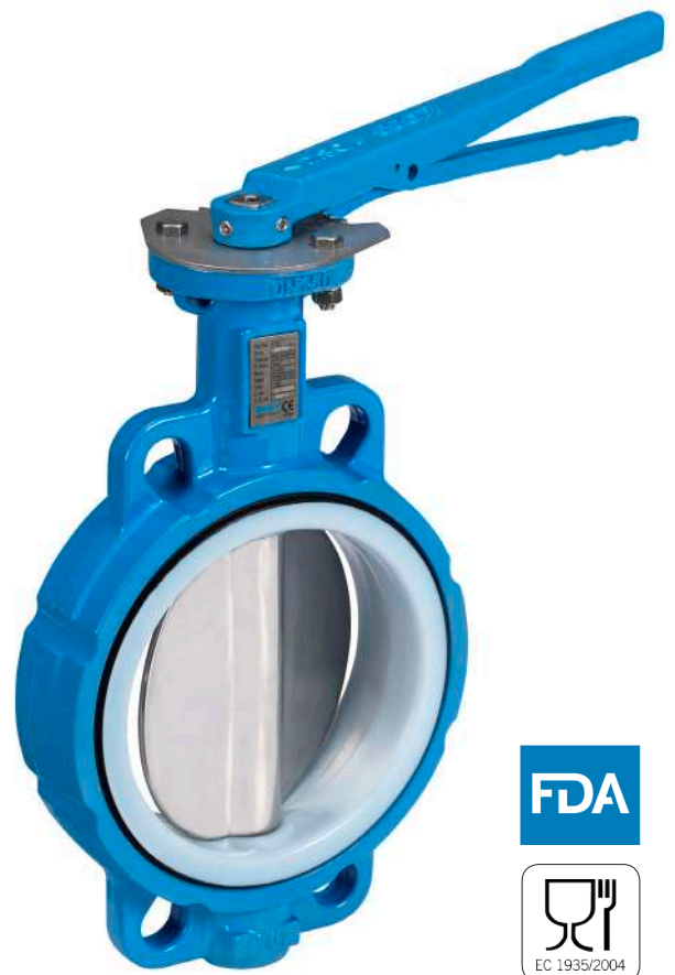
Wafer type with TFM 1600 seat and stainless steel polished disc for food applications Fig. 6731
