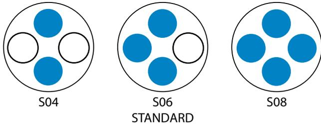
SR-40 and 80 spring return actuators use a minimum of two springs and maximum of seven springs on each side according to the diagram below.
